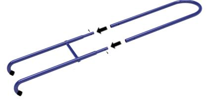
2. Insert screws into the left and right-side holes. *{Philips Screwdriver}*
